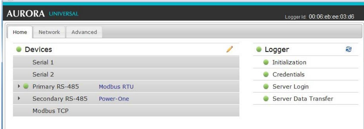
The MAC address (Logger ID) for the Data Logger is displayed at the top of the page. Be sure to write down the MAC address of the Data Logger. The MAC address will be needed later for Asset Registration.
