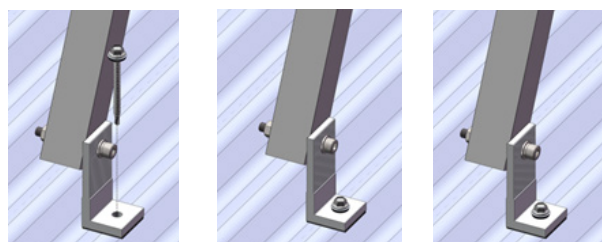
Figure 9 (Tin Foot Rear Leg Installation)
